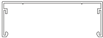
LS311: 75mm WR Glazing Section
